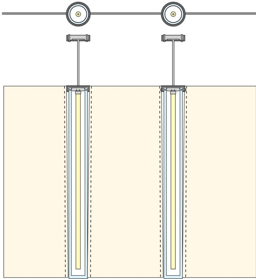
The cross section of two lights shows the construction of the light tube with the fabric which slides over the light and a flap that secures the system. The exploded view shows the assembly of the parts.
