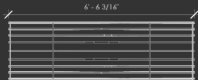
HORIZON PENDANT 6.5' MODULE plan scale 1/2" = 1'0"
